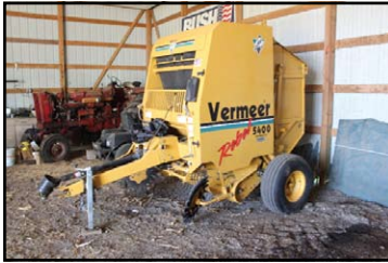
Vermeer Rebel 5400 Round Baler, Accutie, Gathering Wheels, Double Twine Arms, 540 CV PTO, Controller, SN- 1VRV111D421002258, Good Condition
