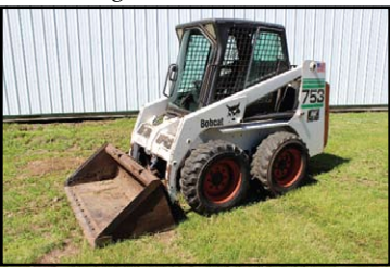
Bobcat 753 Skid Loader, Aux Hyd, Enclosed Cab with Door, Heat, 10.00-16.5 Tires, 60" Material Bucket with bolt on cutting edge, 2750 Hours Showing
