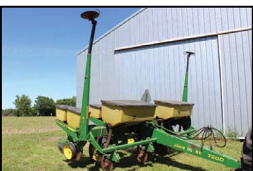
JD 7200 4R40" Planter, Herbicide Boxes, Dry Fert Boxes, Finger Pickup
